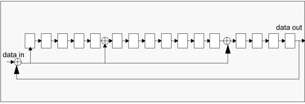
Figure 4-13: CRC16 Generator/Checker
