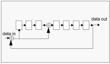
Figure 4-12: CRC7 Generator/Checker
