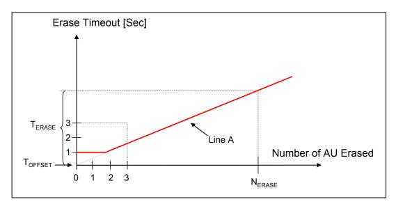
Figure 4-17: Example Erase Characteristics (Case 1 T<sub>OFFSET</sub>=0)
