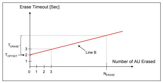
Figure 4-18: Example Erase Characteristics (Case 2 T<sub>OFFSET</sub>=2)
