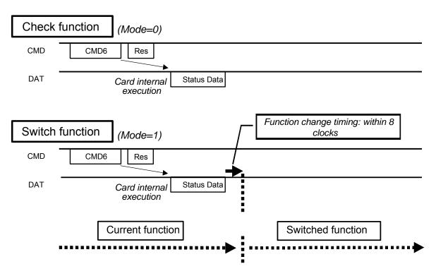
Figure 4-10: Use of Switch Command
