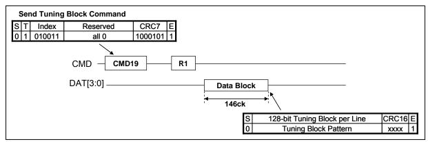
Figure 4-8 : Send Tuning Block Command
