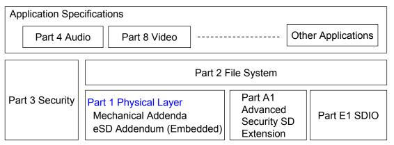
Figure 1-1: SD Specifications Documentation Structure
