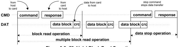
Figure 3-2: (Multiple) Block Read Operation
