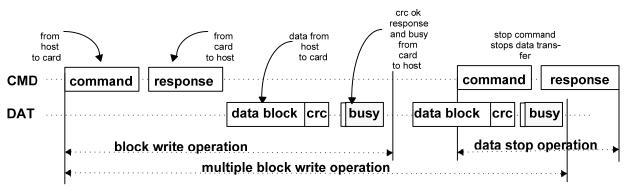
Figure 3-3: (Multiple) Block Write Operation
