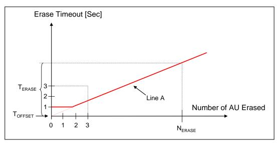
Figure 4-10: Example Erase Characteristics (Case 1 Toffset=0)
