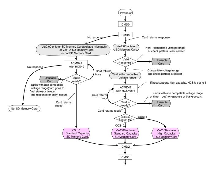
Figure 4-2: Card Initialization and Identification Flow (SD mode)
