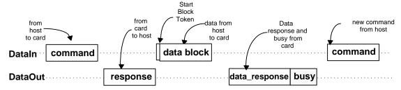
Figure 7-6: Single Block Write Operation
