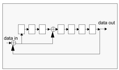
Figure 4-6: CRC7 Generator/Checker
