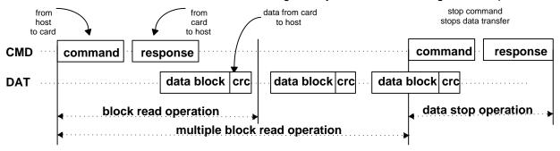
Figure 3-3: (Multiple) Block Read Operation
