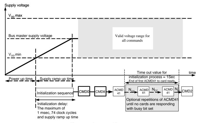
Figure 6-1: Power-up Diagram
