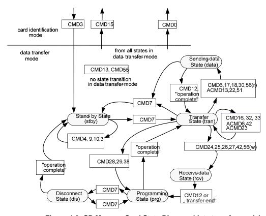
Figure 4-3: SD Memory Card State Diagram (data transfer mode)
