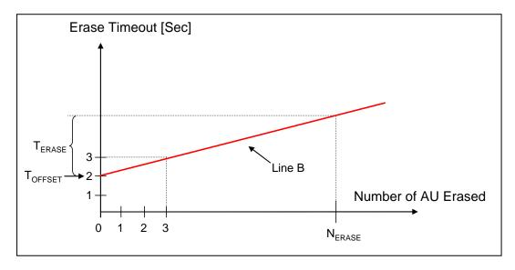
Figure 4-11: Example Erase Characteristics (Case 2 T<sub>OFFSET</sub>=2)
