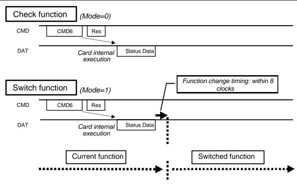
Figure 4-4: Use of Switch Command
