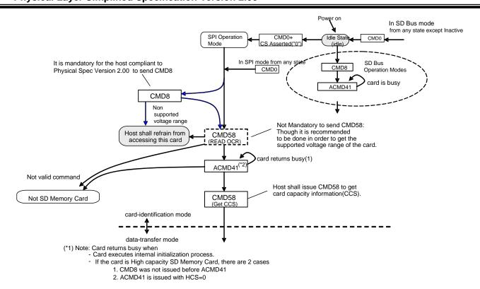
(\*2) Note: 2.1mm SD Memory Card can be initialized using CMD1 and Thin (1.4mm) SD Memory Card can be initialized using CMD1 only after firstly initialized by using CMD0 and ACMD41. In any of the cases CMD1 is not recommended because it may be difficult for the host to distinguish between MultiMediaCard and SD Memory Card.
