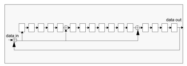
Figure 4-7: CRC16 Generator/Checker
