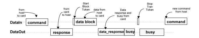
Figure 7-7: Multiple Block Write Operation
